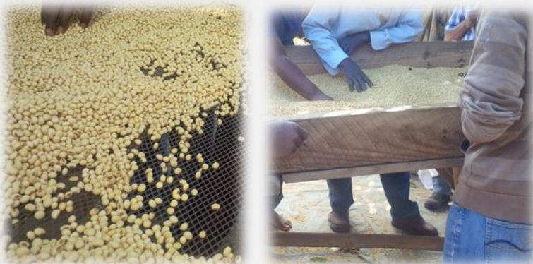
Picture 4: Sieving platform made of wooden materials being used for cleaning soy beans
