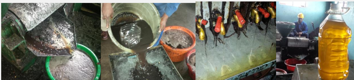
Picture 10: Oil clarification in the process where filtering is a key process step
