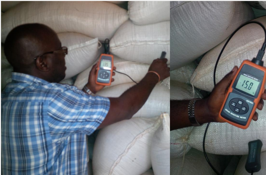
Picture 6: A commercial moisture meter being used to test moisture content for the oil seeds in stock
