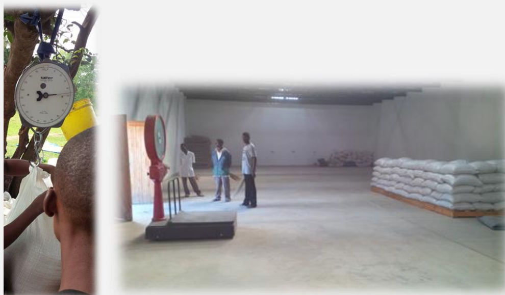
Picture 2: On the right side is a spring scale used for recording weight of farm deliveries at a satellite aggregation center while on the right is the platform scale recommended for warehouse usage.
