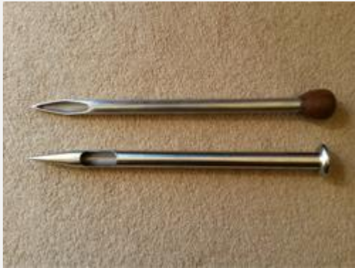
Picture 3: A commercial canular for sampling oil seeds and grain stocks upon receiving them at a storage facility
